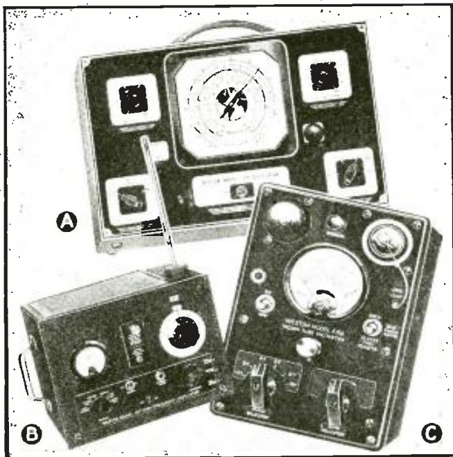
Illustrated here are representative, Weston precision instruments suitable for efficient testing and alignment of frequency modulation receivers. They are identified as follows: A, model 776 oscillator; B, model 787 high-frequency oscillator; C, model 669 V.-T. voltmeter.
